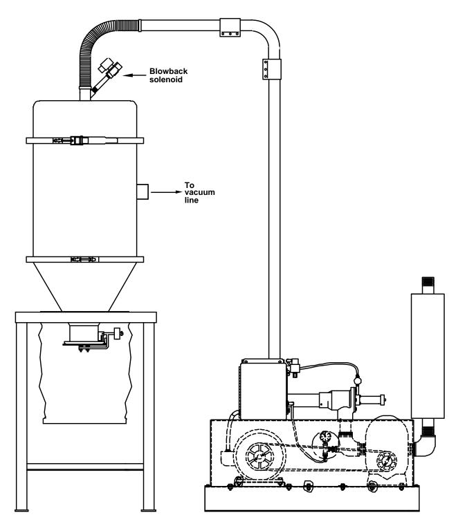
Figure 21: Filter Chamber Installation, Optional Blowback Controller Shown
